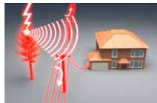
Coupling by radiation
